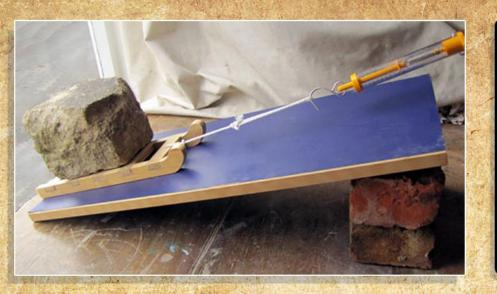
Another way to move a object is to place a sled underneath it and then pull it. Placing the object on top of a sled helps to create much less drag when pulling the object.
